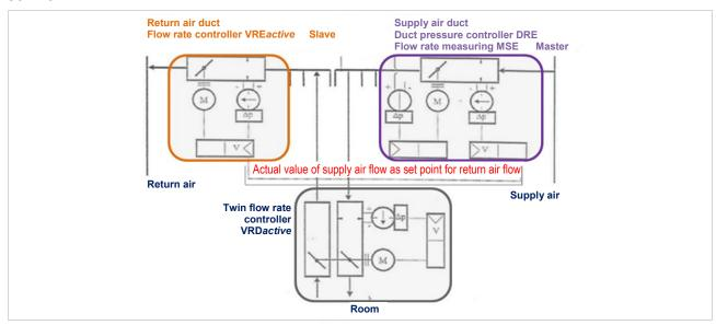
Control diagram: Integration of the flow rate controller
