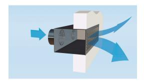
Displacement air diffuser
