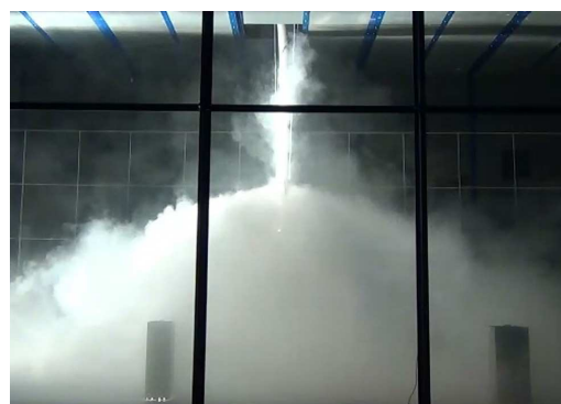
Room flow in case of cooling, up to 3 m high, \Delta t = -5\text{ K}
