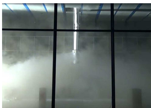
Room flow in case of heating, up to 3 m high \Delta t = +10\text{ K}
