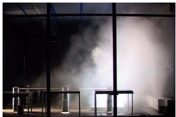
Example of room air flow: VFC with special fan insert for mixed air/displacement air
