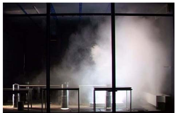
Example of room air flow: VFN with special fan insert for mixed air/displacement air
