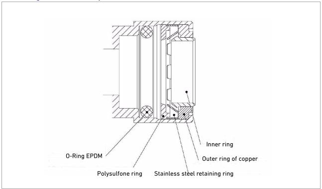
Tube connection of plug-in fitting and bright copper tube according to EN 1057 and RAL 641/1 or suitable brass or red brass socket.
