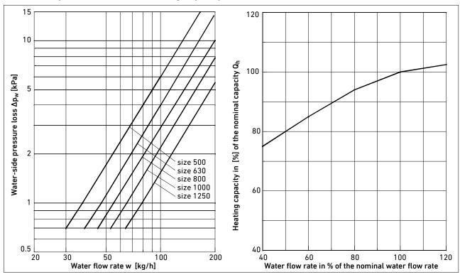
**Note:** The minimum water flow rate must not be lower than 20 % of the standard flow rate for cooling, and 40 % for heating, considering the water-side pressure compensation.
