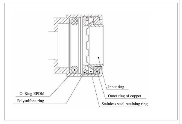
Tube connection of plug-in fitting and bright copper tube according to EN 1057 and RAL 641/1 or suitable brass or red brass socket.
