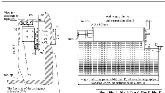
partition plate is supplied detached. To avoid short-circuits between the air intake and air outlet the unit will have to be insulated against the facade.
