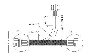
Hose without insulation. For insulated hoses, dimensions will change accordingly.
