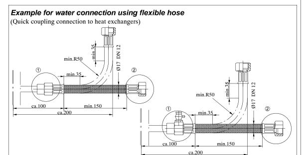
Hose without insulation. For insulated hoses, dimensions will change accordingly (10 mm Armaflex insulation).
