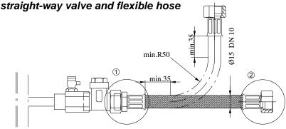
Hose without insulation. For insulated hoses, dimensions will change accordingly.
