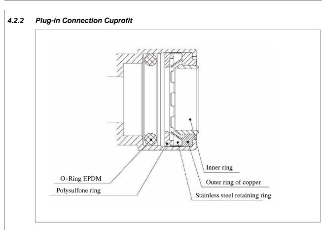
Tube connection of plug-in fitting and bright copper tube according to EN 1057 and RAL 641/1 or suitable brass or red brass socket.
