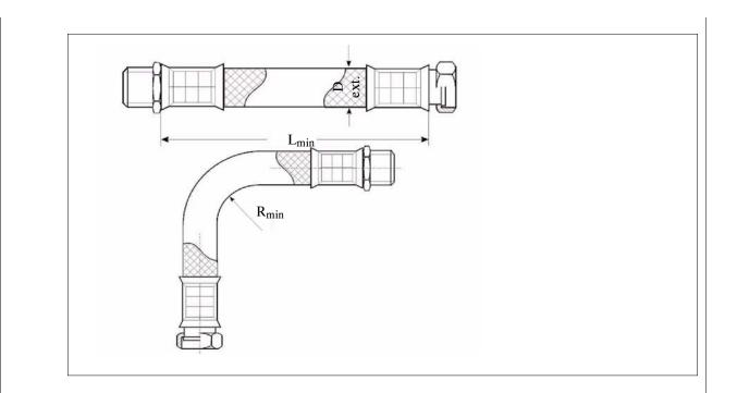
Armoured hose Oxystop up to +70 °C (diffusion inhibiting, marked through weaved-in blue strip) Armoured hose EPDM up to +93 °C (vapour permeable, not marked)
