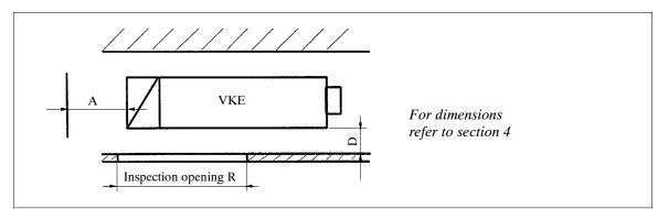
R: Inspection opening to grant access to the unit (especially the electric and the water connections) for maintenance and installation must be provided
