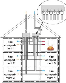
Figure 2 >> In the figure, when the fire creates overpressure (in fire compartment 6 in the figure), the back draught damper in the intake air duct
