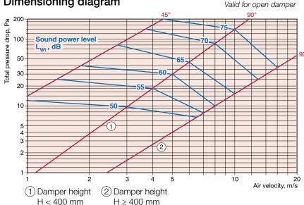
The speed is calculated on the damper's gross area, i.e. a BSK6R - 400 x 400 has a gross area of 0.16 m<sup>2</sup>.
