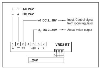
**CAUTION!** When connecting several VAV devices to the same transformer, it is important that all system phases are connected to  $(\sim)$  and all system neutrals are connected to  $(\bot)$ .
