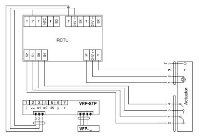
When connecting several VAV-devices to the same transformer, it is important that all system phases are connected to ( $\sim$ ) and all system neutrals are connected to ( $\perp$ ,
