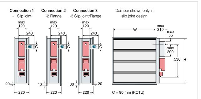
RABR-VAP for mounting in combination with RBVG is supplied with Slip joint/Flange type 3 connector. RABR-VAP with height dimensions 250, 450, 650 and so on are supplied with raised slip joint or flange.
