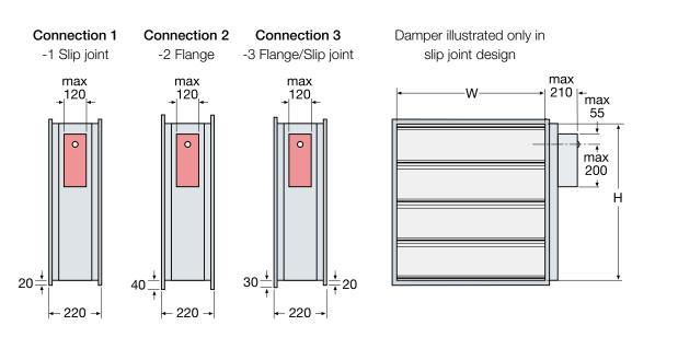
RABRR for installation in combination with RBVG supplied with connection type 3 Slip joint/Flange. RABRR with height size 250, 450, 650 etc. is supplied with a raised slip joint or flange connection.
