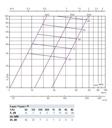
The adjustment position, shown in the diagram, represents the amount of open horizontal rows on the back side of the product.
